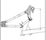
The height of the crank can also be adjusted. Slacken the screw connec-451 tion of the bottom bracket and screw it back again at the desired height.
