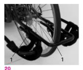
sed knee bend does not lead to contact with the drive crank. There must be a minimum gap of 5 cm between the heel and the floor. You will need this clearance for travelling round bends. After any adjustment work, ensure that all screws are tight (see page on torque).
