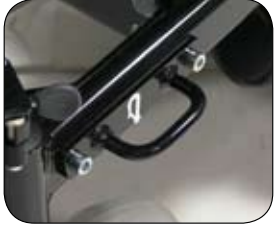
Front and rear tie down hooks for use with 4 point tie down system.
