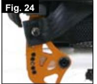
The lap belt is fitted to the wheelchair as shown in the illustrations. The seat belt comprises 2 halves. They are fitted using the existing seat stay retaining bolt fitted through the eyelet on the belt. The belt is routed under the rear of the side panel. (Fig. 24)
