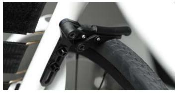
Ergonomic compact wheel locks. Minimalist, easy to lock. Can be screwed direct to the frame (on 0 and 3 degree wheel camber only). Also suitable for 'quads'. (Option)
