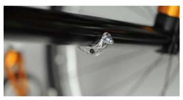
Wheel camber options with optimal wheel alignment. Visual guide ensuring optimal wheel alignment (toe in/toe out) when you fit the 3 and 6 degree camber options. Zero degree camber available as standard.
