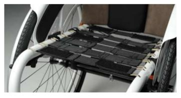
Innovative clip upholstery, combined with lighter seating and back materials. This option provides the minimal solution for adjustable seating, is elasticated for profiling and still allows easy centre of gravity adjustment.
