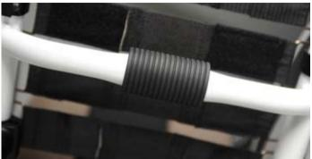
An oval ergonomic hand grip ensures balanced lifting of the chair from the cross bar for easy car transfers. An additional oval hand grip is available on the back rest as an option (see Electron pack).
