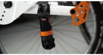
Quick, simple, rigid, light centre of gravity adjustment. Loosen two screws each side and slide the COG along the frame. No need to remove skirt-guards. 7.2 cms of infinite adjustment for fine balance.
