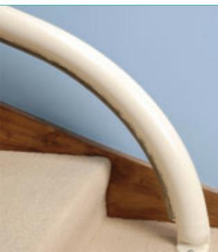
Handicare's tight-fitting drop nose rail can save having to fit a hinged track at the bottom of the stairs. A wall length of only 250mm is required.
