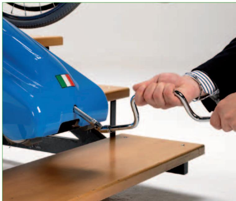
Double, electrical and mechanical lock, of the steering bar connection to the motor casing
