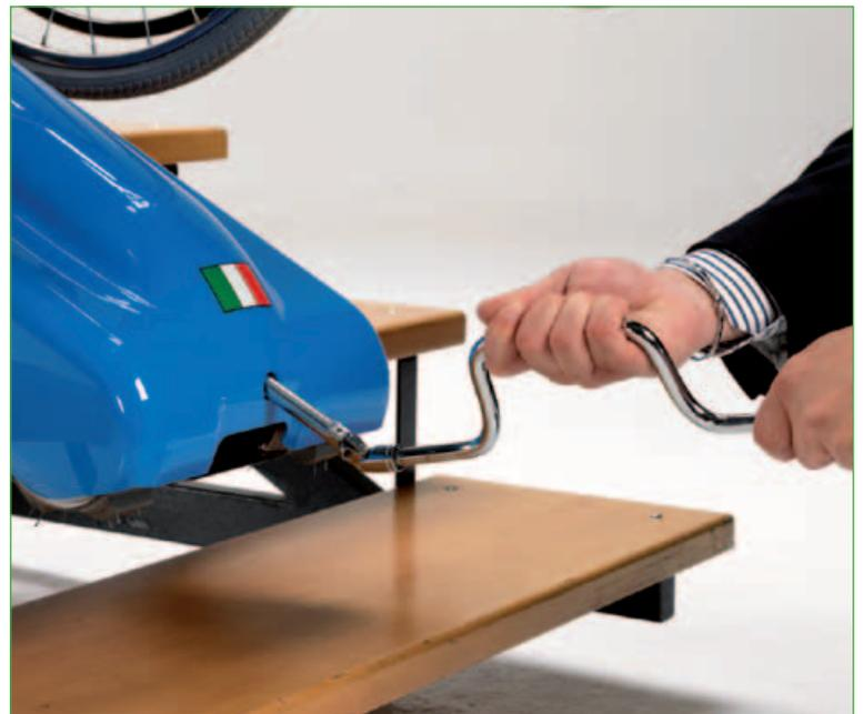
Double, electrical and mechanical lock, of the steering bar connection to the motor casing
